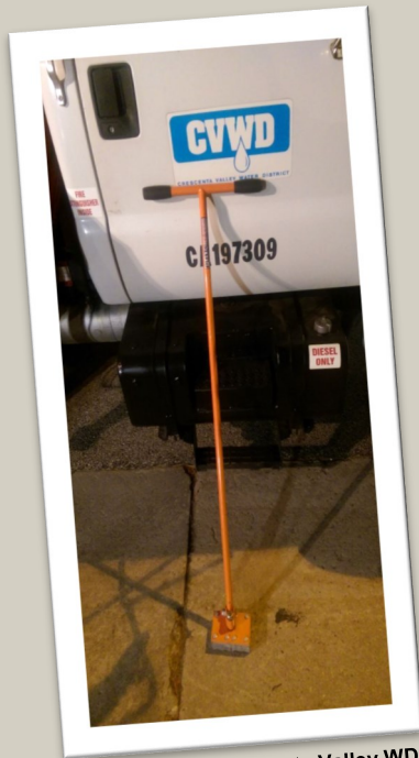
Bryan Jones, Crescenta Valley WD Tool with magnets to move heavy road plates.
