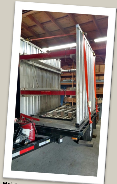
Maintenance Dept., Humboldt Bay MWD A trailer was fabricated to hold trenching and shoring equipment.
