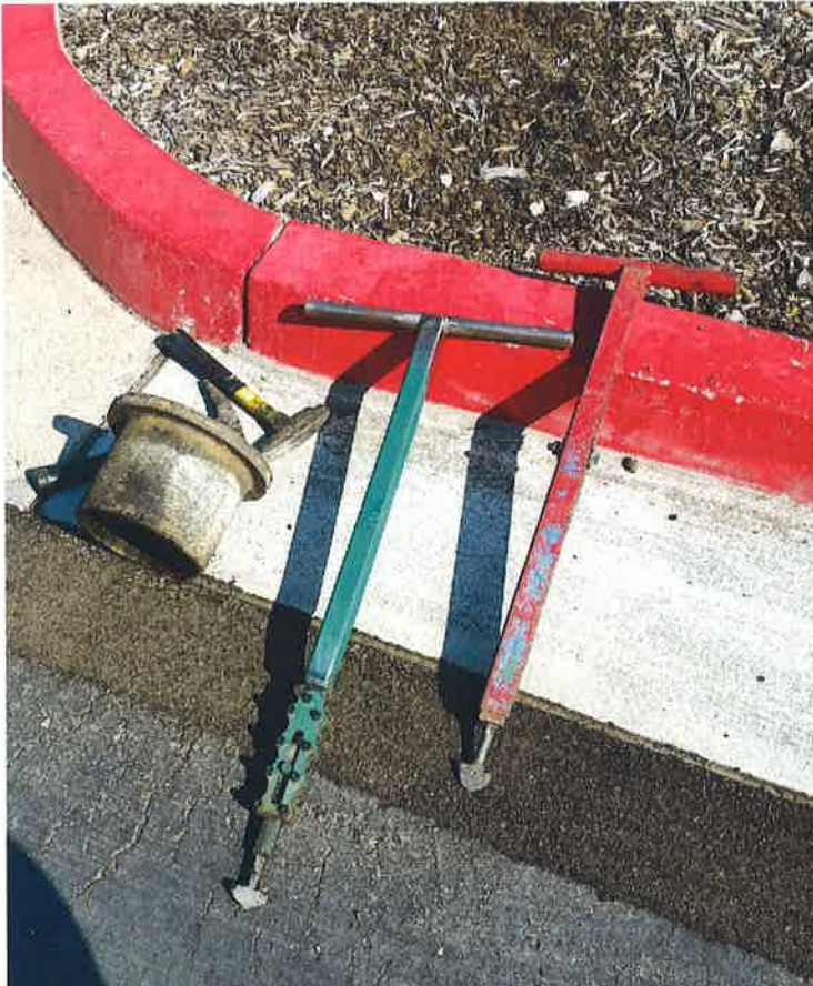
Rock pick hammer, final and initial lifting tool design
