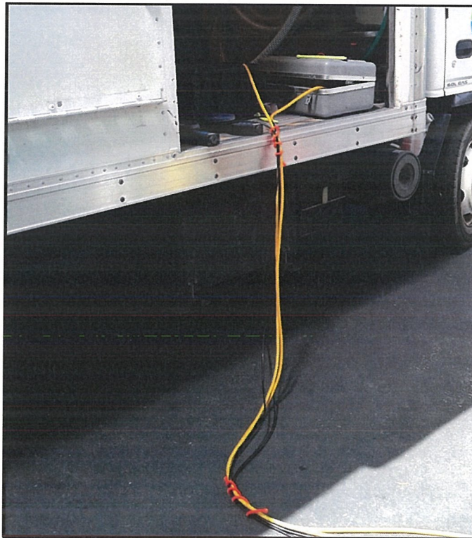
After: Improved Electrical Cord Management (Help Prevent Tripping Hazards)
