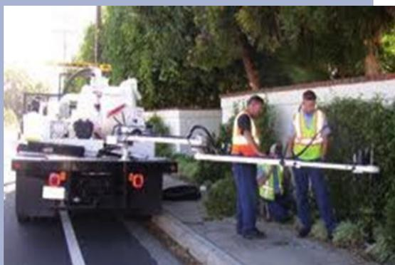
**Figure 3. A Truck-Mounted Valve Turner**
