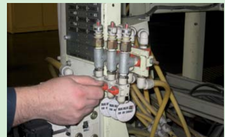
Bleeding air pressure by opening a valve
