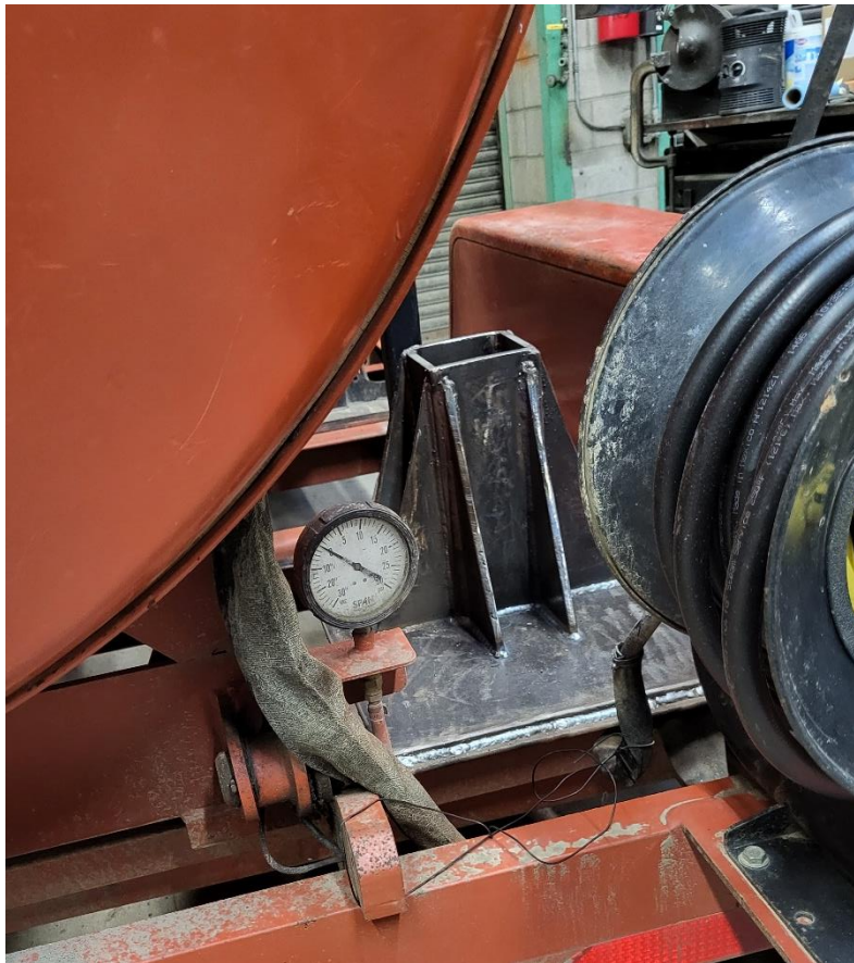
Mounting bracket installed
