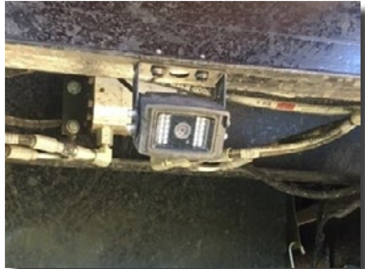
Rear camera on the excavator
