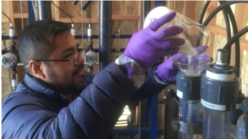
Ricardo Medina, an Orange County Water District research associate, loads ion exchange resins into a treatment system to filter out PFAS toxins. The district is testing 14 different products to determine the best to remove the carcinogenic chemicals from dozens of Orange County groundwater wells. (File photo courtesy of the Orange County Water District)
