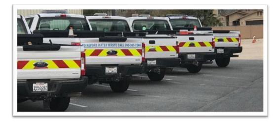
It is recommended that the strip of tape be between 36 inches (bottom), and 48 inches (top), above the road with a minimum tape width of 6 inches.
